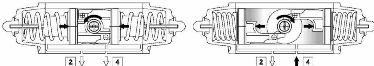
d) This double acting GD special version, with the pistons rotated and extra long adjustment screws, limits the actuator/valve travel in the open position and is used when the valve should never be totally open, but limited up to 45% of its capacity.
