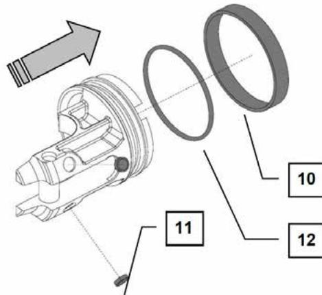
D) When the components are disassembled, they should be properly cleaned, and wear checked prior to being greased and reassembled. In case the sealing parts are too much worn out use new parts from the spare parts kit.
