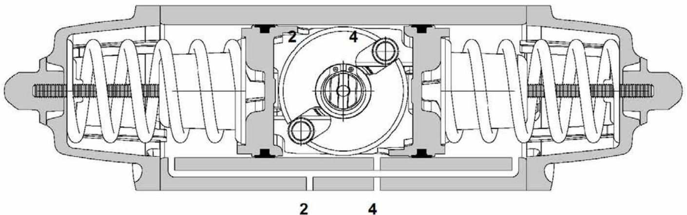
The port 4 is in connection with the intermediate chamber and when pressurised the drive shaft rotate counter clockwise to open.
