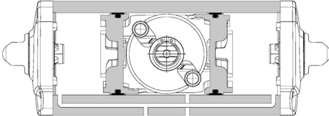
The port 2 is in connection with the cylinder side chambers, supplying the pressurised air in port 2 the standard Double Acting actuator drive shaft rotates counter clockwise to open, while the port 4 is in connection with the intermediate chamber and when pressurised the drive shaft rotates clockwise to close.
