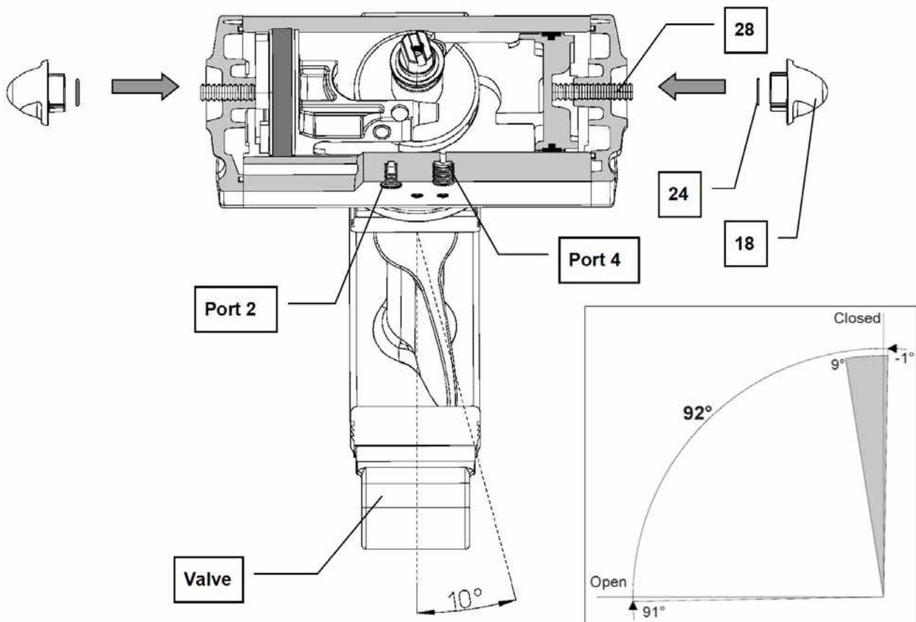
**b) GS Spring return Fail to Close stroke adjustment instruction.**
