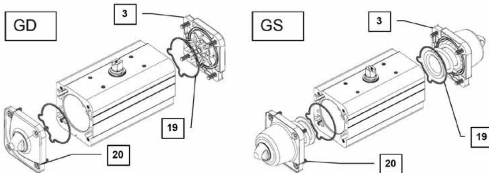
**Caution.** The Spring Return end caps cartridges (Parts N° 3 + 18+24+19+23+22+21) are a safety device, where the preloaded spring is set to avoid the dangerous spring jumping. Do not release the screw (part N° 21) to remove the spring from its seat, this operation must be done by ACTUATECH technician only.
