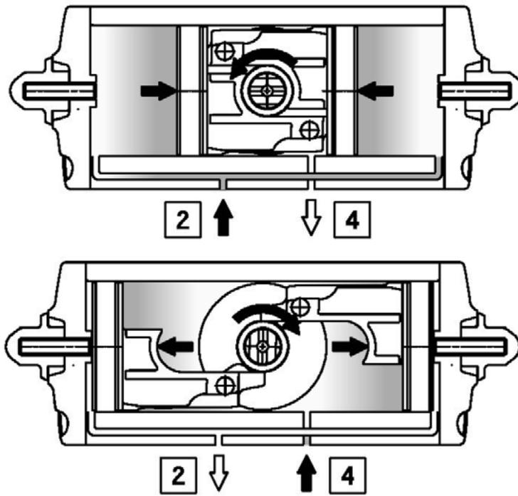
**Simple Acting Spring Return fail to close operation cycle (GS Type).**
