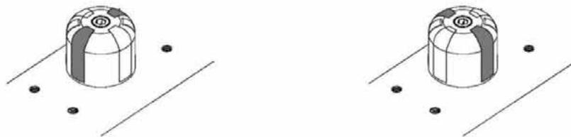
**Simple Acting Spring Return fail to open operation cycle.**
