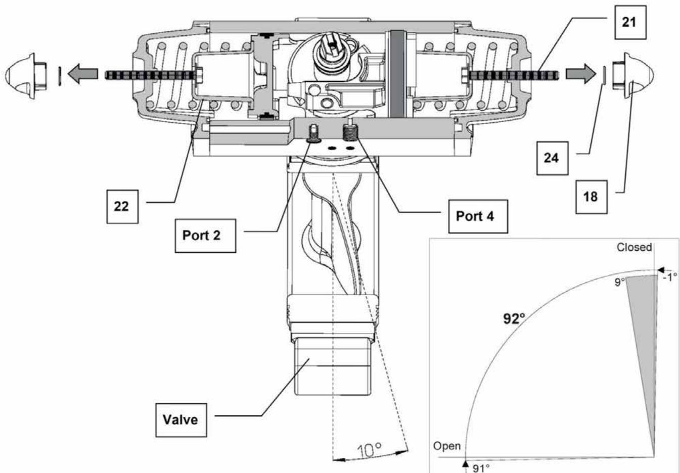
**\*\*\*WARNING.** The Spring Return close adjustment is not a mechanical stop that act against the pistons travel or the shaft rotation, but the screws limits the spring travel and the pistons without any force standstills. In this condition the shaft is not stopped and theoretically could be moved to the total closing position, adjustments of closing and opening cannot be performed both. ACTUATECH standard stroke adjustment is max 10°, special longer screws are available on request.
